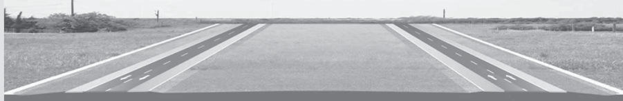
Phase 2: Add Second Two-Lane Frontage Road and Convert Phase 1 to One-Way Operation
