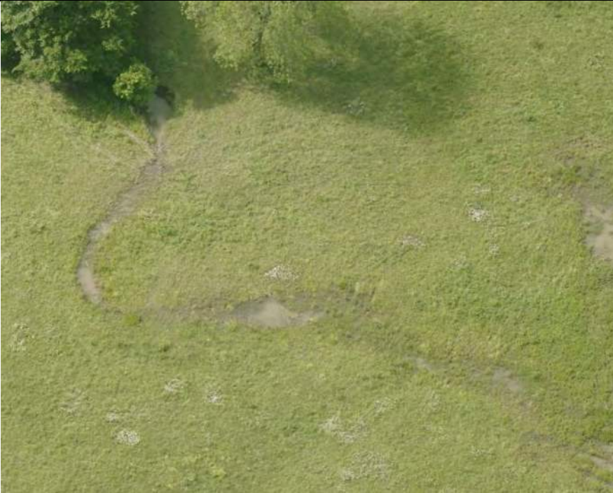
Photo 159. Representative aerial photo (Pictometry 4/27/17) of Intermittent Stream Water Feature 359 and Water Feature 360. Note the sharp shift from vegetated, pasture swale to channelized, water- filled stream channel. This is the result of ditches constructed upstream that cut off the native channel.
