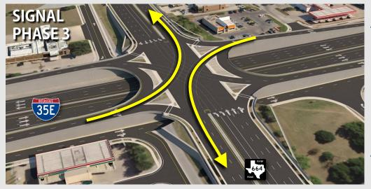
Left turn Traffic from the Frontage Roads to FM 664. This phase will also allow right turn yield from the IH35E to FM 664. Through movements will utilize a bypass roadway. A **S**ingle **P**oint **U**rban Interchange (SPUI) is an innovative intersection design that improves mobility by allowing vehicles to travel more quickly, safely and efficiently through an intersection.
