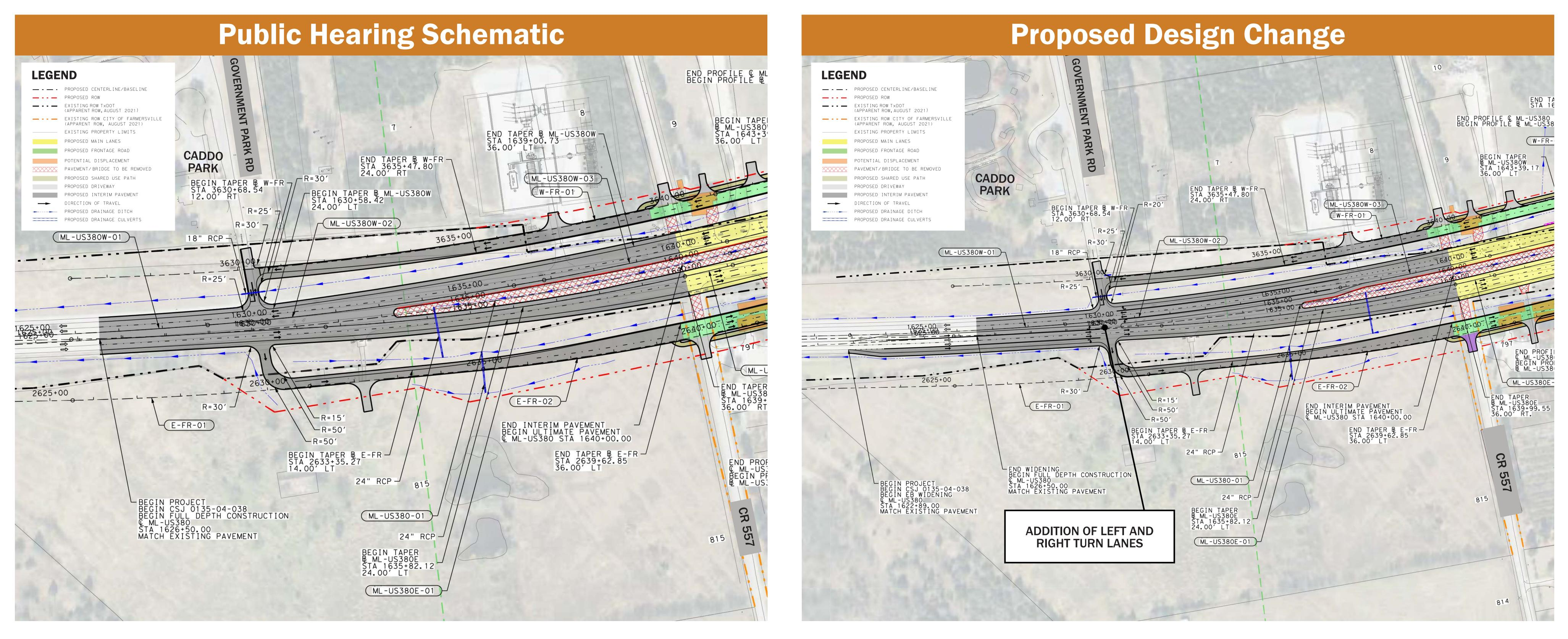
To increase the safety of the transition from the existing section with a two-way left turn lane to a divided median, turn lanes would provide a safe refuge for traffic turning onto Government Park Road. This change increased the total project length from 7.86 to 7.93 miles.
