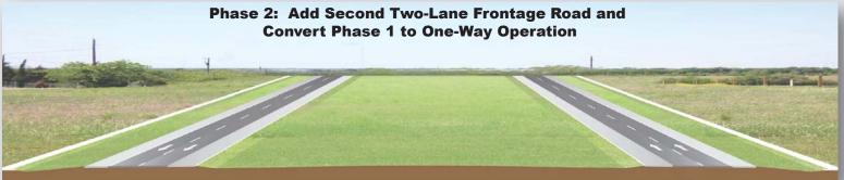
As traffic warrants and funding becomes available, PHASE 2 would involve the construction of the second two-lane frontage road and the conversion of the two-way frontage road built in Phase 1 to a one-way operation. This frontage road facility would include:
