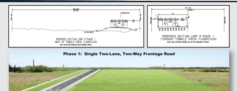
**PHASE 1** would construct a single two-lane, two-way frontage road, and would also acquire the proposed ROW to accommodate the frontage roads and the future ultimate access-controlled mainlane facility. This frontage road facility would include:
