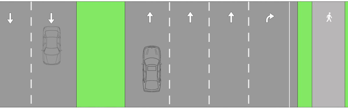
• Three 12-ft lanes in each direction with a 18-ft wide median and curbs, and 2-ft curb offsets. 10-ft wide shared use path with American Disabilities Act curb ramps in both directions. Urban roadway right-of-way (ROW) width is 200-ft (usual).
