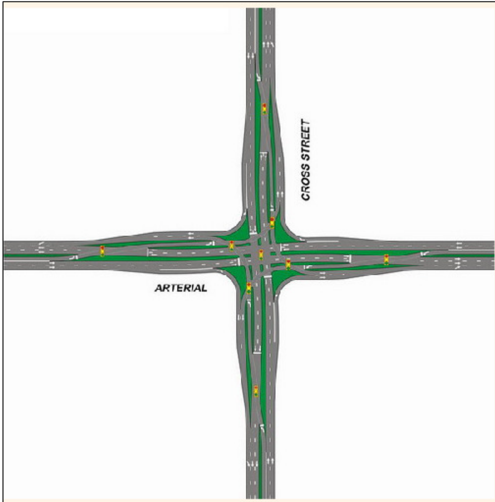
Figure 17: Concept Design of CFI Intersection Geometric Improvement
