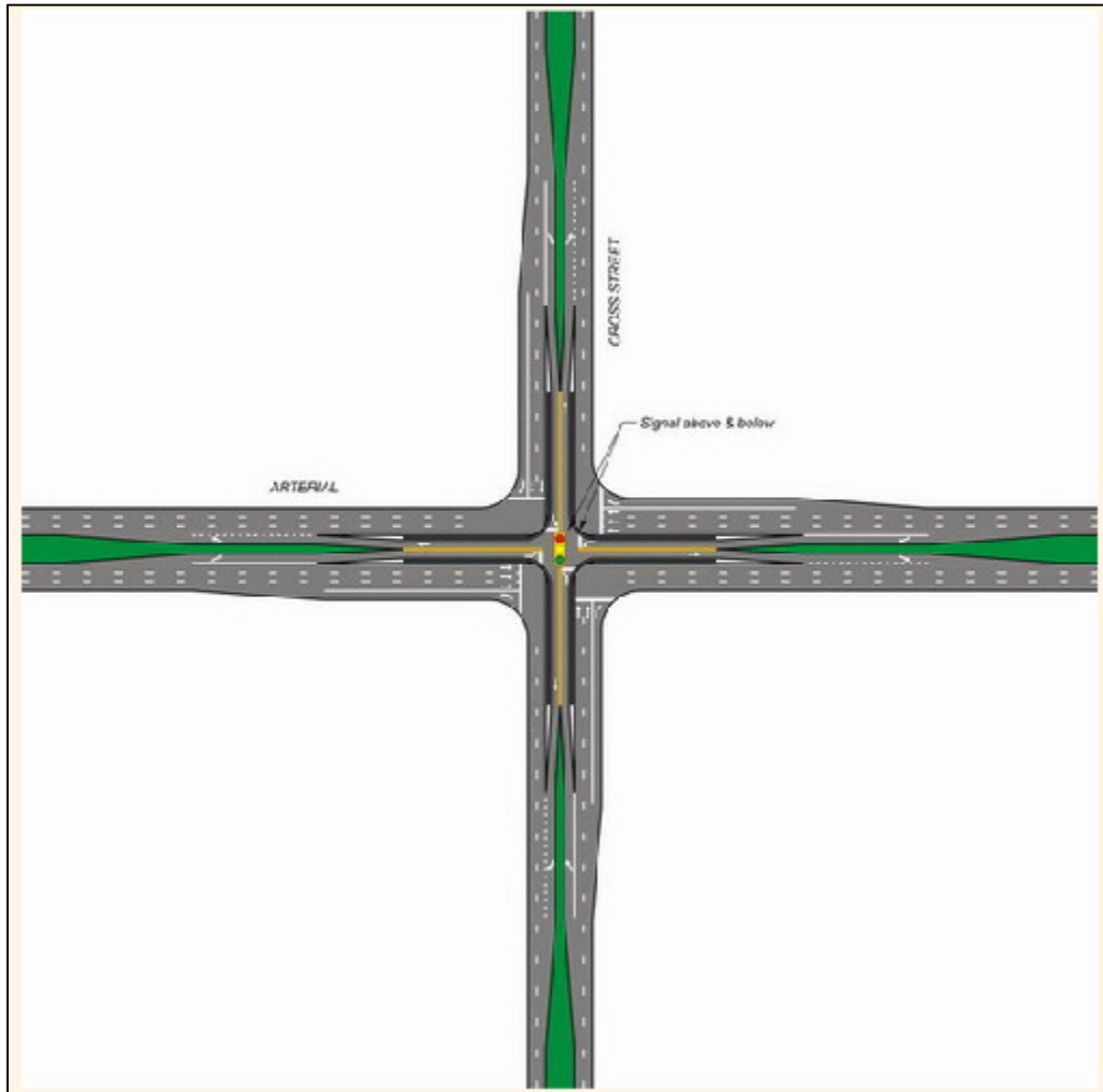
Figure 18: Concept Design of Grade Separated Left Turn Intersection Geometric Improvement
