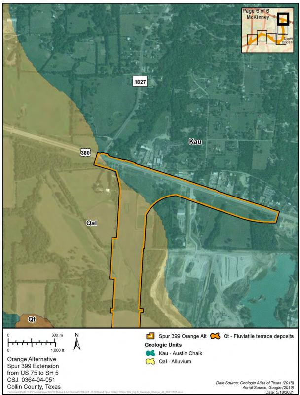
Figure 3a. Subsurface geology of the project area for the Orange Alternative.
