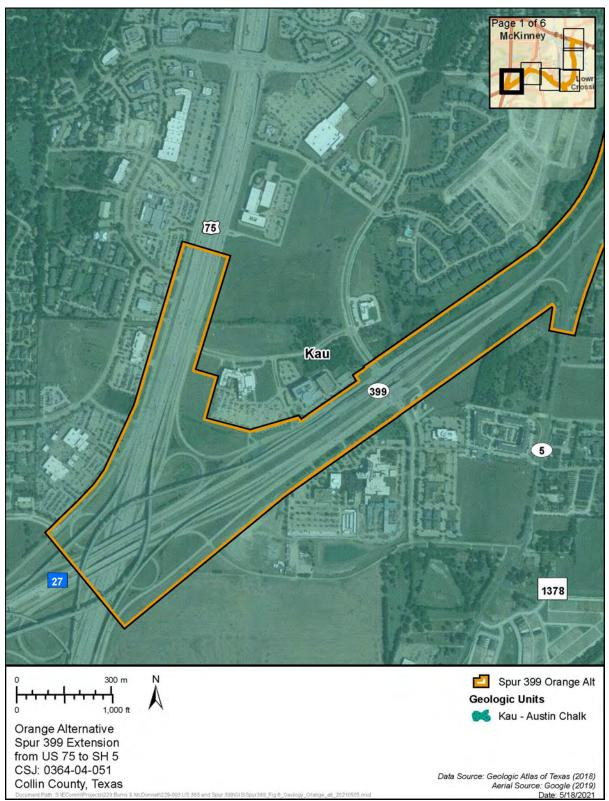
Figure 3f. Subsurface geology of the project area for the Orange Alternative.
