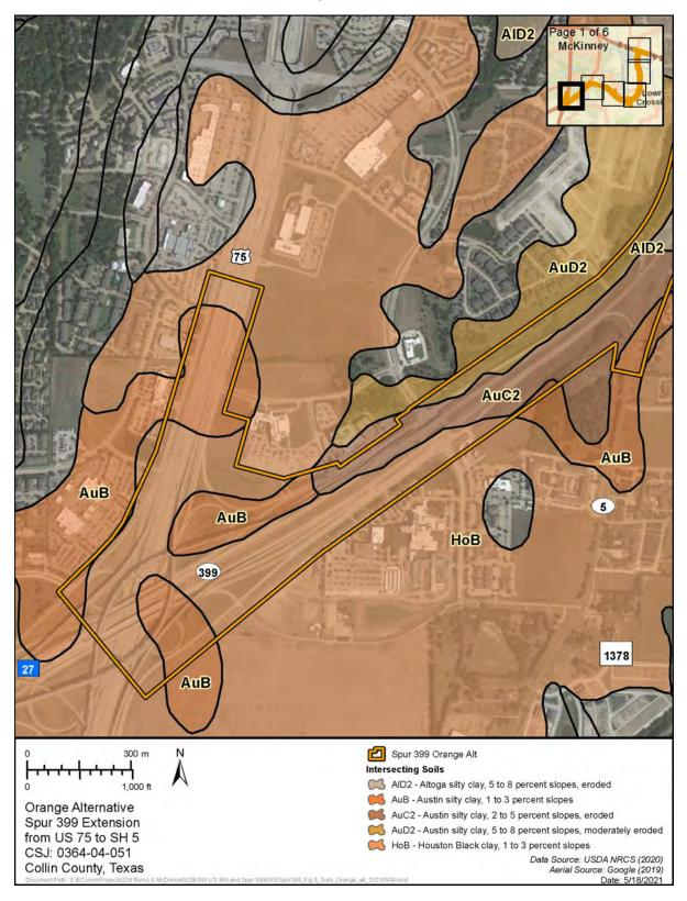
Attachment 6b: Soils Map for Spur 399 Orange Alternative.
