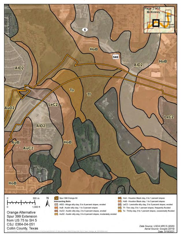
Attachment 6c: Soils Map for Spur 399 Orange Alternative.
