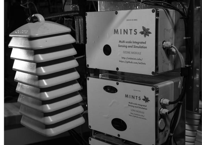
The MINTS-AI team is working on a set of air sensors that take in data about temperature, pressure, humidity and more to measure air quality at different points in Dallas. The group seeks resources and funding to create more of the sensors.
