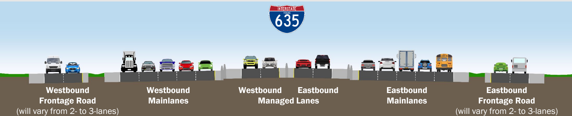
Proposed Typical Section (I-635 from Luna Road to I-35E)
