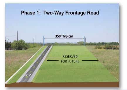
Phase 2 will construct the other side of the paired frontage road. Each side of the frontage road will be converted to oneway operation. The median will be left open for the future Phases 3 & 4. Phase 1 will consist of One Two-Way Frontage Road. The right-of-way (ROW) for all phases will be purchased during Phase 1. The decision regarding which side will be built first would be made in the next study.
