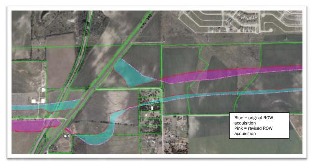
Exhibit 4: Loop 9 shift at SH 342 by converting loop ramps to jug handles
